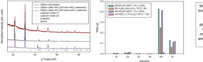
Shows the importance of knowing which phases are present in shredded material before attempting purification – Nitric acid appears to remove the spinel phase while sulfuric removes the layered phase.
