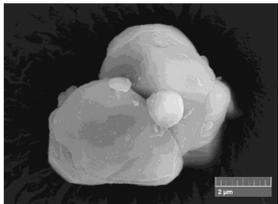
Figure 1: SEM image of NMC622 single crystal powder.
