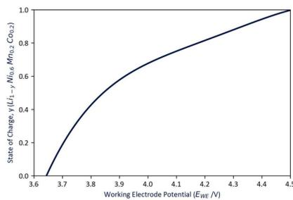
Figure 5: Curve fitting working electrode potential to state of charge for NMC622 based on data from a previous C/20 cycle.
