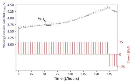
Figure 3: Working electrode potential and current in first 180 hours of NMC622 GITT cycle.
