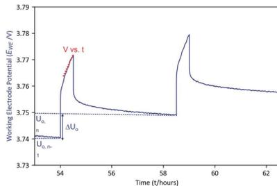
Figure 4: Zoom in on potential/time GITT plot showing a single pulse and relaxation with how the open circuit voltage  $U_o$  was obtained.
