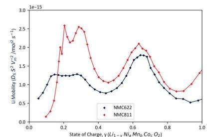
Figure 6: Calculated Li mobility versus state of charge for NMC622 and NMC811
