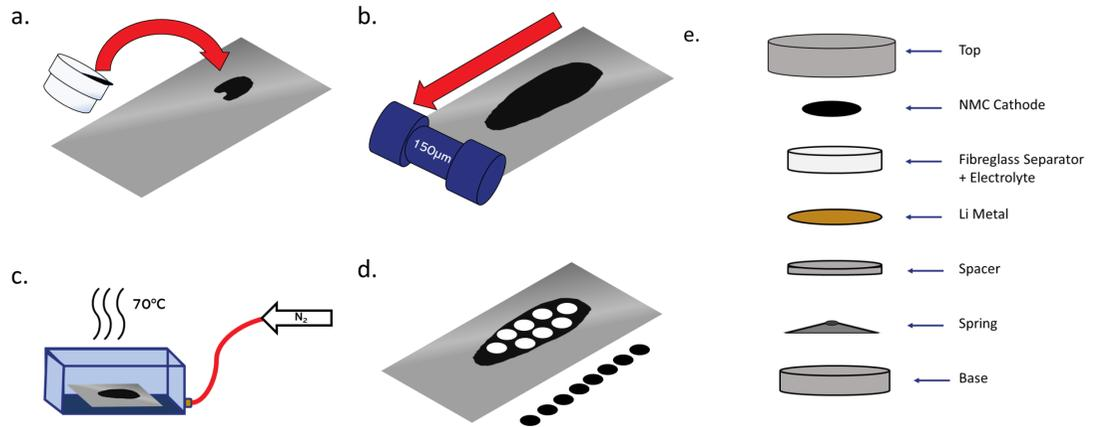
Figure 2: Electrode casting steps (a-d) and coin cell configuration (e).
