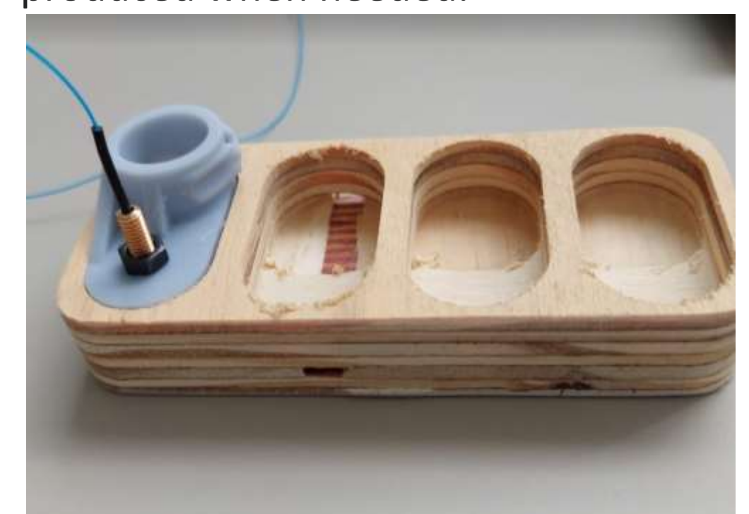
Fig 4: The final version of the pin alignment jig manufactured by CNC machining from wood laminate.
