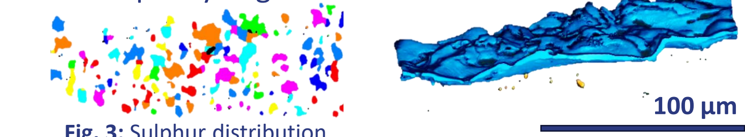
Fig 4: Sulphur (yellow) and Li 2 S (blue) in discharged "155" cell
