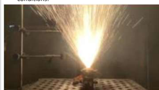
Fig. 1: Li-Ion Battery under Thermal Runaway
