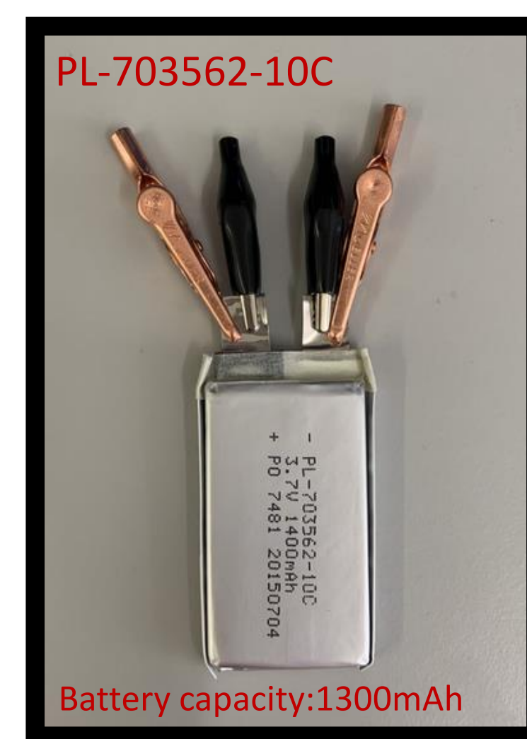
Figure 3 - Image of an example pouch cell used in this study
