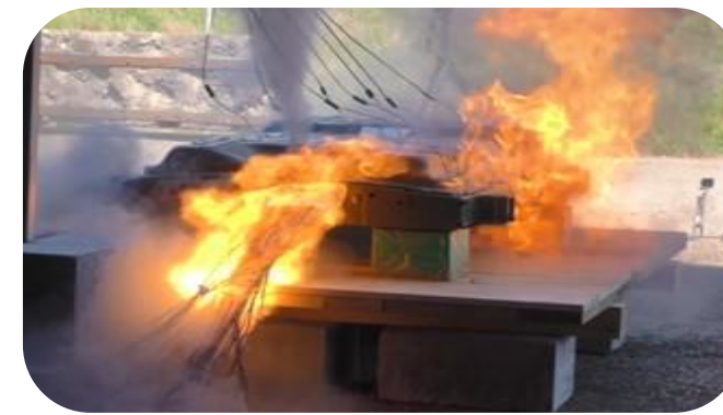
Fig.1. Overcharge of the pack, resulting in thermal runaway
