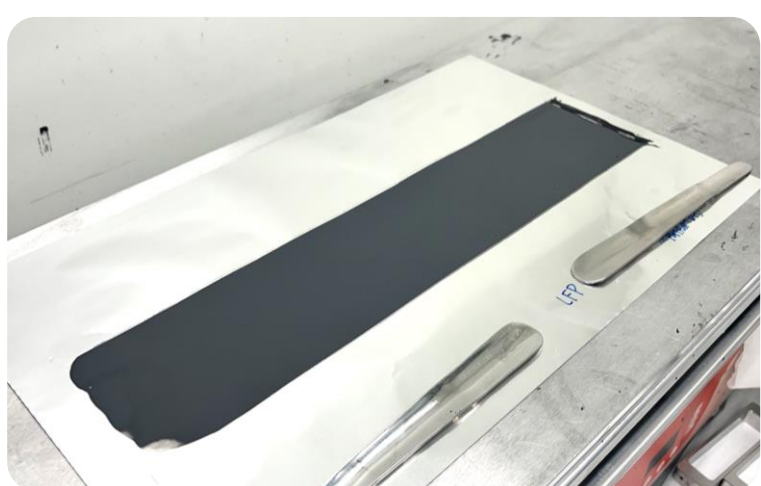
LFP slurry coating on Al foil
